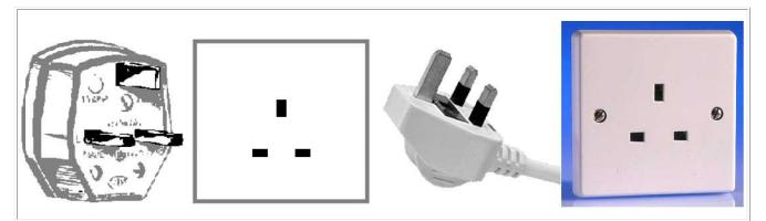
This plug has three rectangular prongs that form a triangle. British Standard BS 1363 requires use of a three-wire grounded and fused plug for all connections to the power mains (including class II, two-wire appliances). British power outlets incorporate shutters on line and neutral contacts to prevent someone from pushing a foreign object into the socket.
